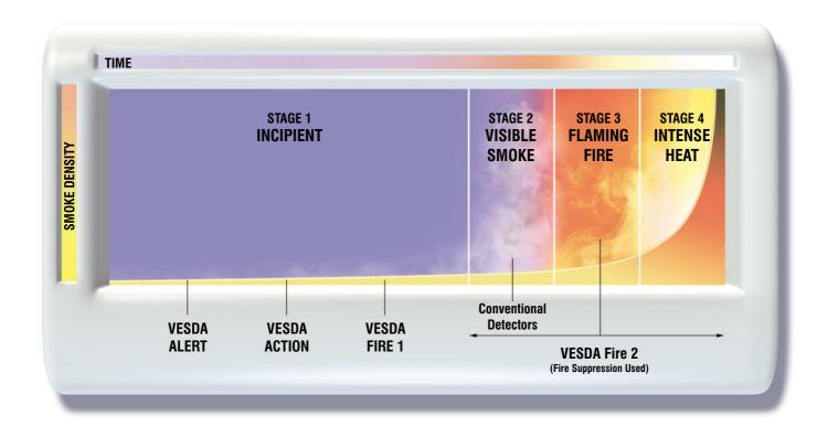
All escalating fires have four stages: Incipient (pre-combustion), Visible Smoke, Flaming Fire, and Intense Heat. This chart shows the progression of fire over a time period. Note that the incipient stage of smouldering fires provides the widest window of opportunity to detect and control the spread of fire, before it takes hold causing major damage and disruption. VESDA can be configured to generate multiple alarms within this window.
