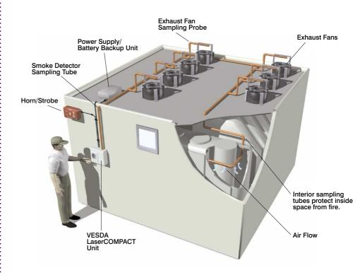
The same process of continually drawing air through a standard pipe network can also be applied to small, single environments including critical process tools. VESDA LaserCOMPACT, which is specifically designed for areas less than 500 sq.m (5000 sq. ft), is shown as a cost effective approach to very early warning smoke detection.
